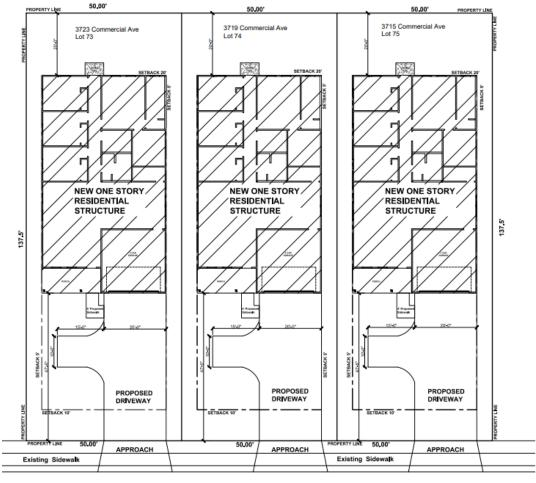
PERMANENT VEHICULAR TURNAROUND SHALL BE PROVIDED ON EACH LOT TO PREVENT A VEHICLE FROM BACKING ONTO THE ROADWAY.
