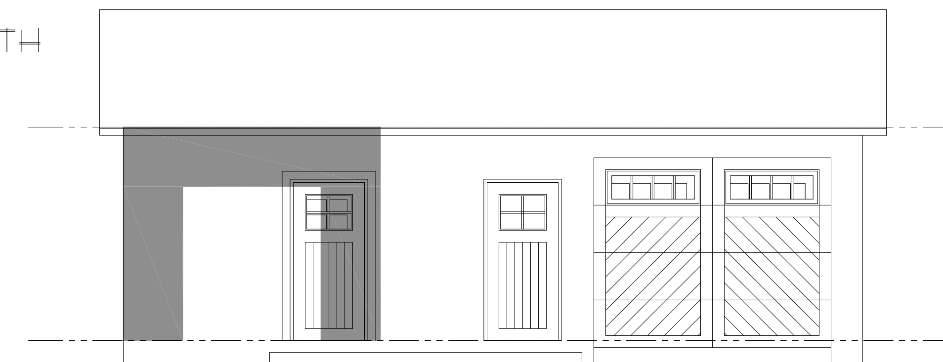
5 NORTH ELEVATION THERMAL ENVELOPE LOCATION SCALE: 1/4"=1'-0"
