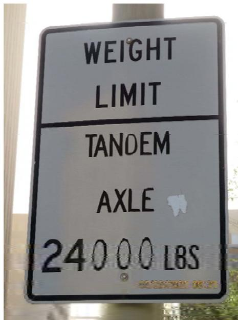
*Figure 21: Weight limit sign for bridge*
