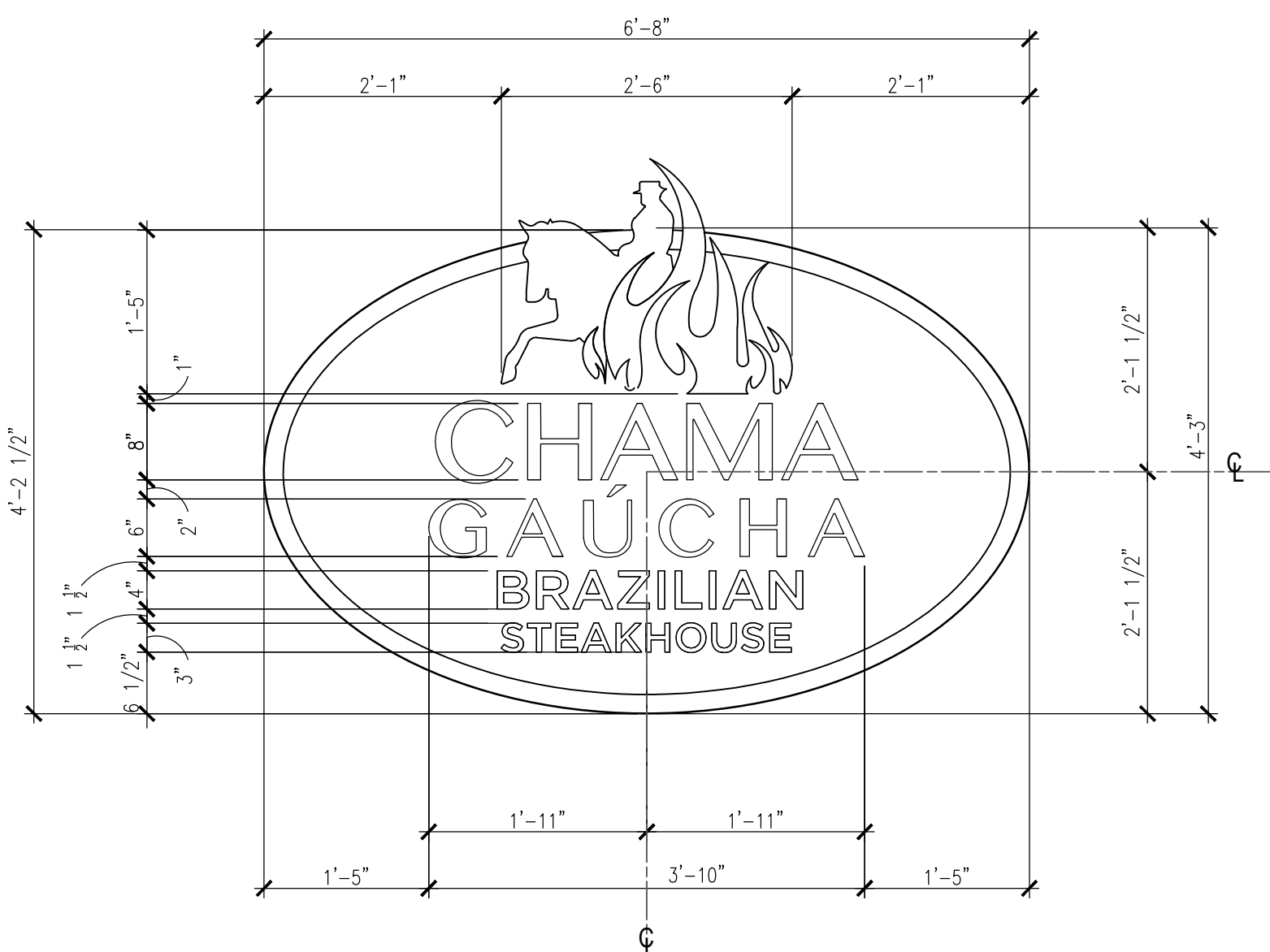
4 ENLARGED SIGN ELEVATION A201 SCALE: 3/4" = 1' - 0"
