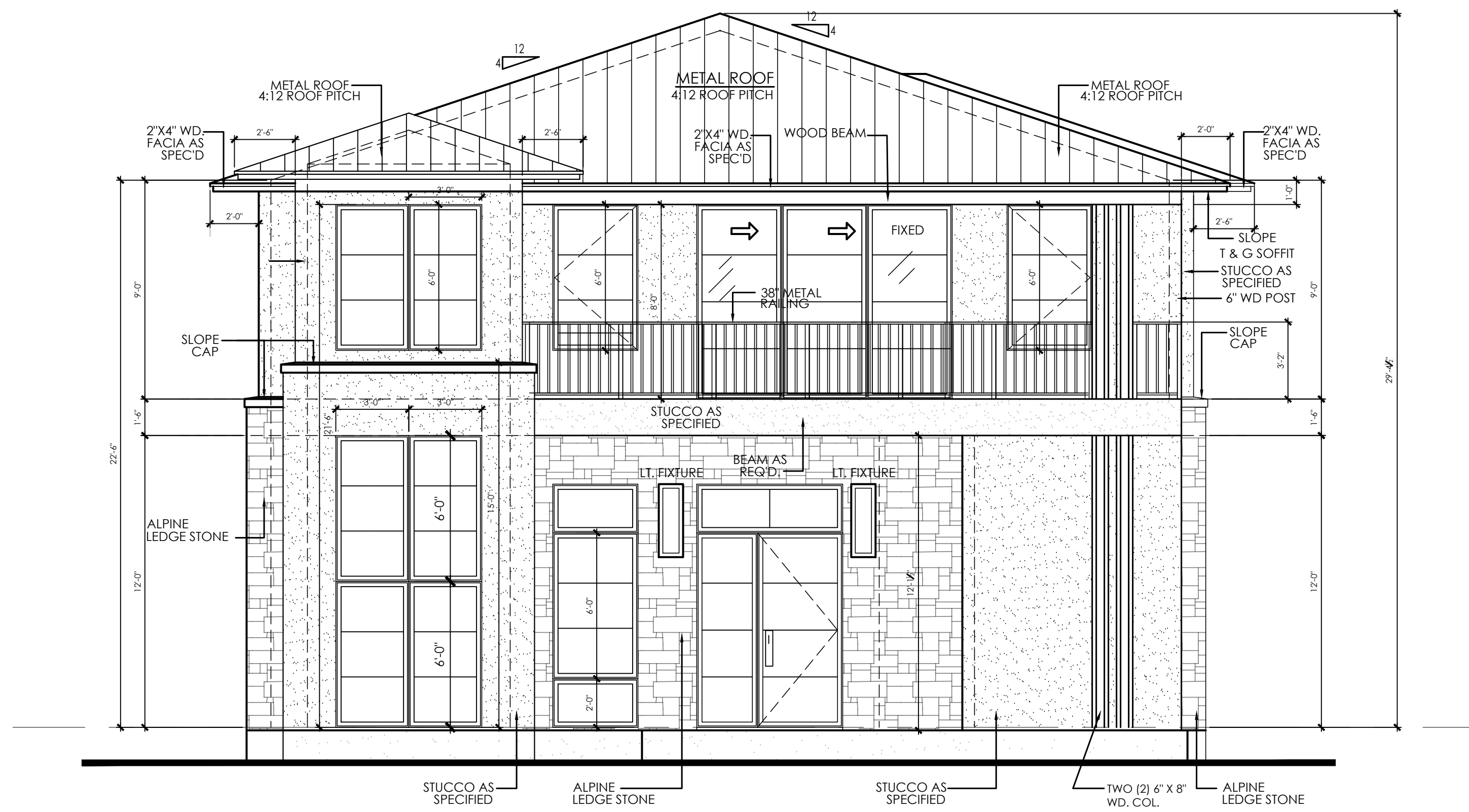
1 FRONT ELEVATION SCALE: 1/4" = 1'-0"
