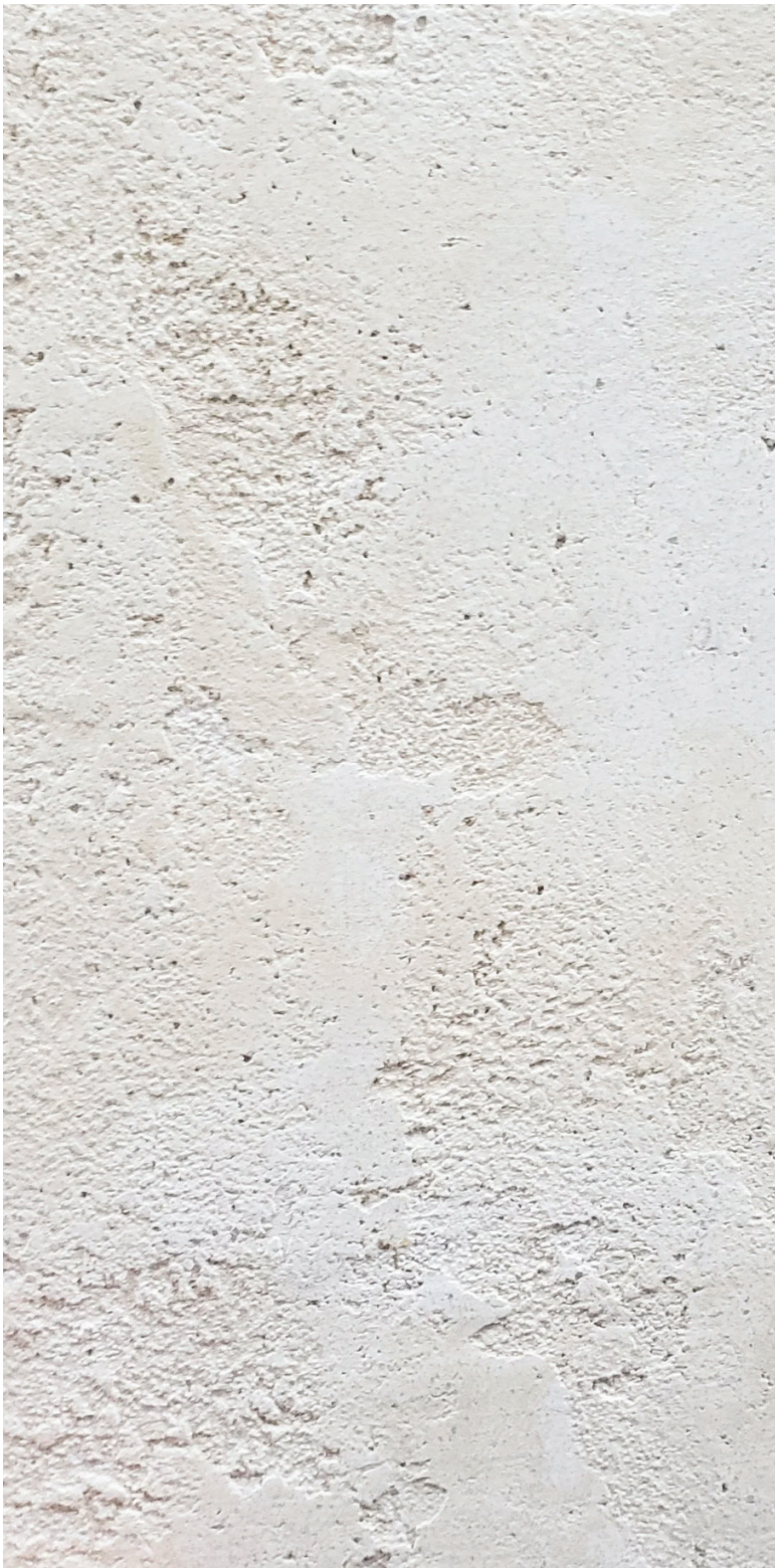
Close-up of stucco top coat made of limestone, marble dust and sand by Vasari. Color to be off-white/ light grey.
