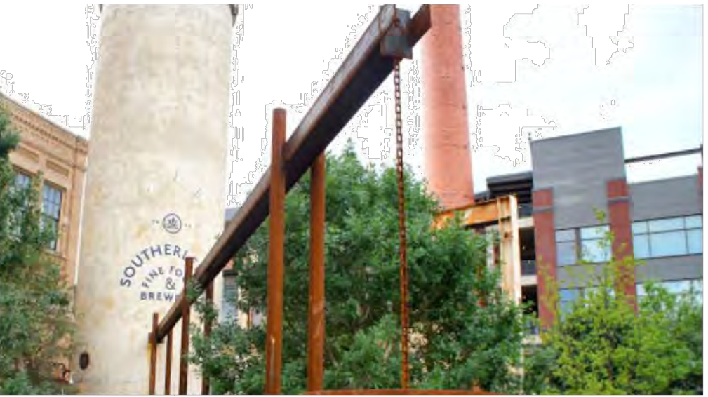
OVERHEAD AQUEDUCT TO DIRECT HOTEL RAINWATER AND BUILDING CONDENSATE INTO LID INLET
