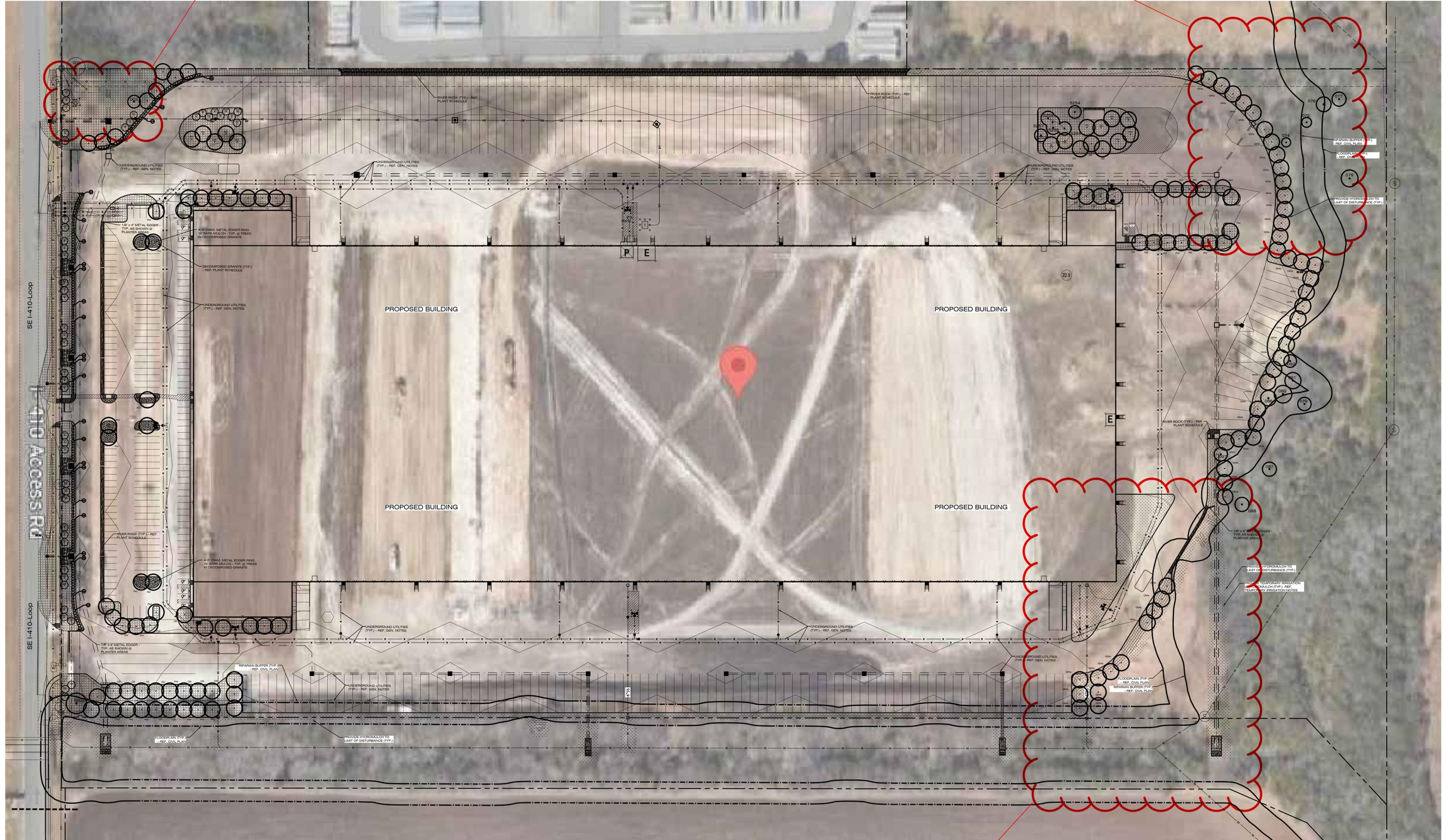
Instead of removing trees where the storm-drain pipe will be installed contractor took a shortcut and graded the entire area clouded removing trees in ESA
