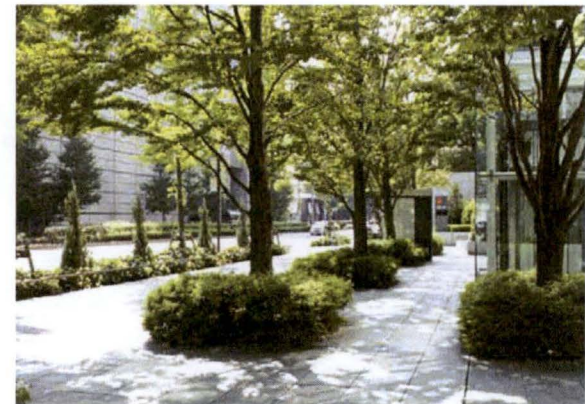
Figure 2.6b: Trees and light-colored paving to reduce heat island effect
