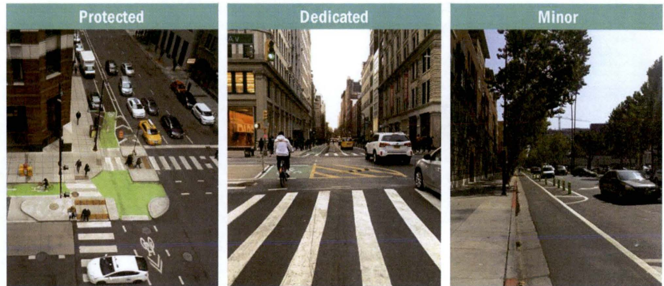
Figure 5.9: Various types of intersection design elements. Source: NACTO
