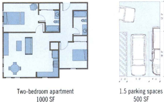
Figure 4.11a: Comparison of required parking and apartment size
