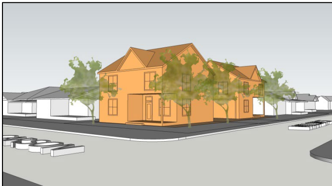
This proposal includes an increase in building scale at a corner location and appropriately responds to each street frontage. The buildings are separated into masses that are compatible with other buildings in the context area.
