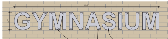
2 ENLARGED ELEVATION DETAIL 1" = 1'-0" NEW GYMNASIUM SIGN
