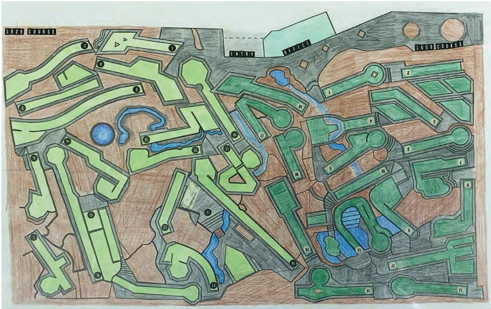
Image 9. Excerpt of a 2013 topographic survey of Cool Crest Miniature Golf showing the overall plan. The original course (left in light green) has geometrically shaped greens whereas the c. 1959 course (right in dark green) has rounded greens and hardscapes and more varied topography. (Source: Frontier Surveying Company)
