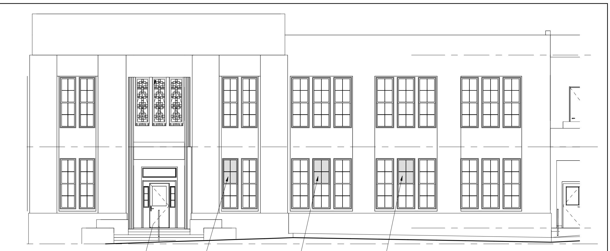
DETAIL C. SOUTH FACADE ALTERED WINDOWS WITH VENTS; REPLACE WINDOWS WITH SALVAGED SASHES
