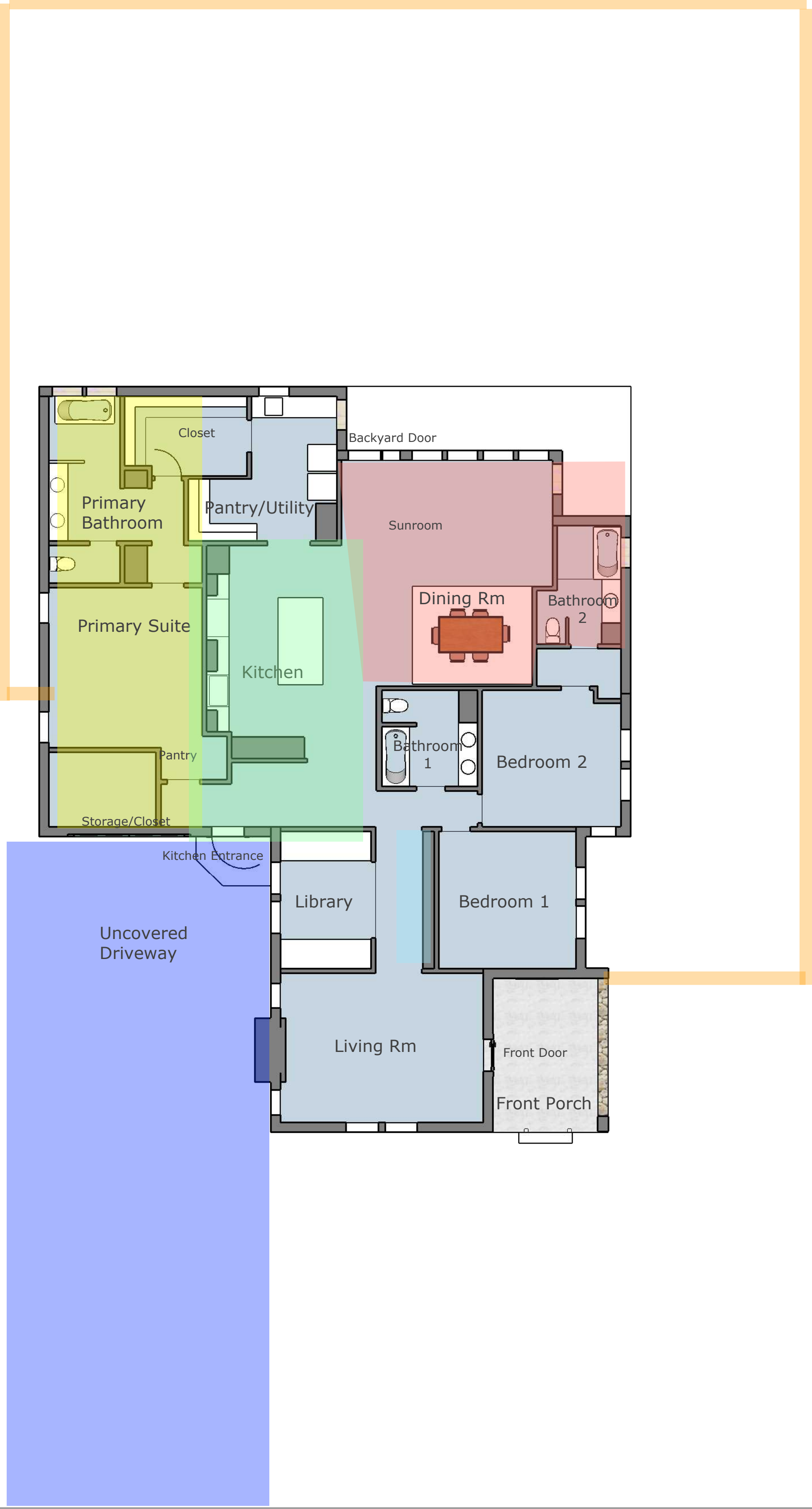
Proposed Design Floor Plan (shown with Property Bounds) SCALE: 1/8" = 1' (1:96)
