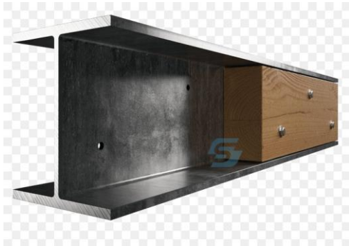
I-BEAM FLITCH BEAM DETAIL @ REAR PORCH
