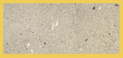
Stone Pavers Limestone, Mocha 20" x 40" , 3" thick Approved materials from 2A to complete Alamo Plaza
