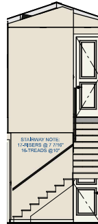
4 STAIRWAY DETAIL 2 SCALE: 1/4"=1'-0"
