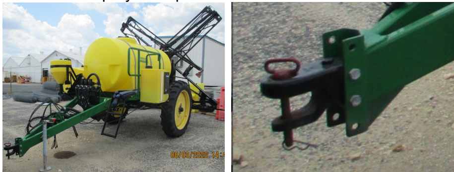
Left photo is the 2009 Schaben Pro 1010. Right photo is clovis hitch for the supplied lunette eye. Pictures are for illustrative purposes only.
