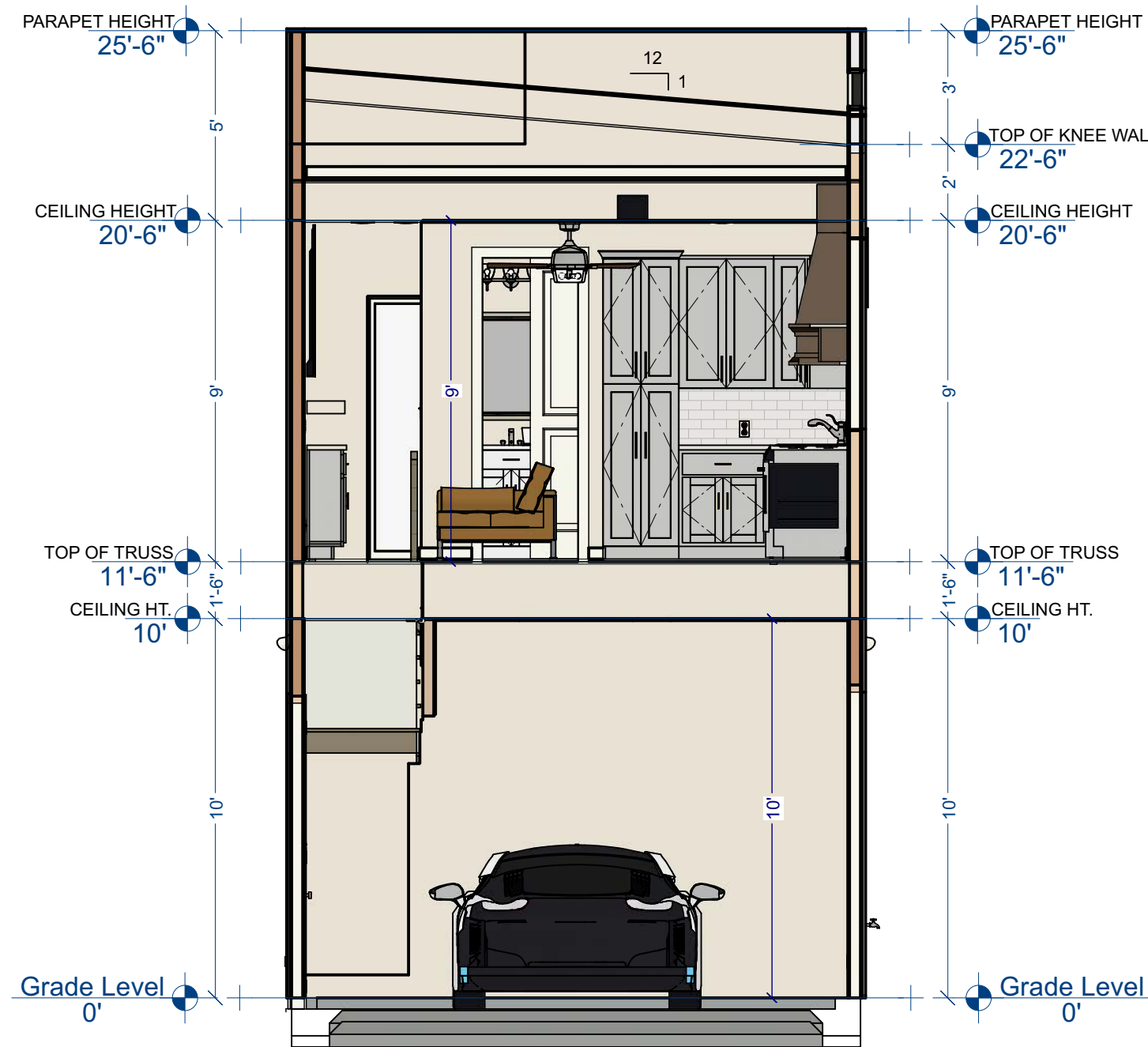
1 CROSS SECTION SCALE: 1/4"=1'-0"
