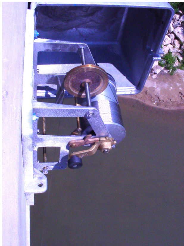
Detail of a wire weight gage
