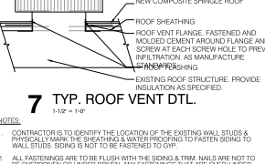
7 TYP. ROOF VENT DTL. 1/2" = 1'-0"
