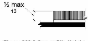
Figure 302.2 Carpet Pile Height
