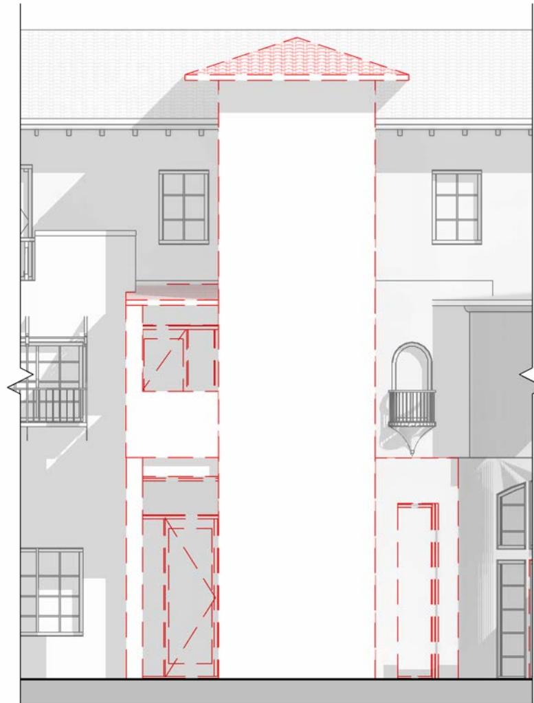
SOUTHEAST ELEVATION - ELEVATOR WALL INFILL 2 1/8" = 1'-0"
