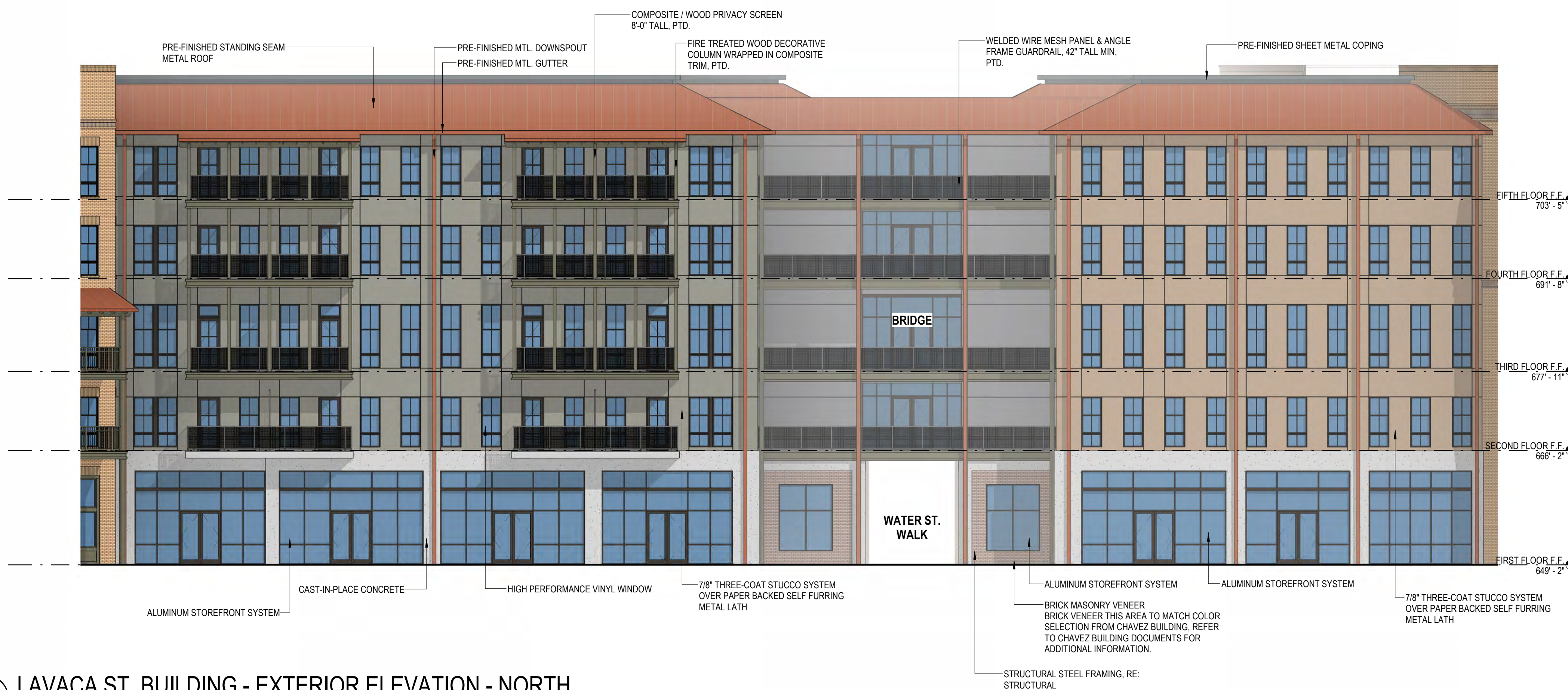
4 LAVACA ST. BUILDING - EXTERIOR ELEVATION - NORTH 3/32" = 1'-0"
