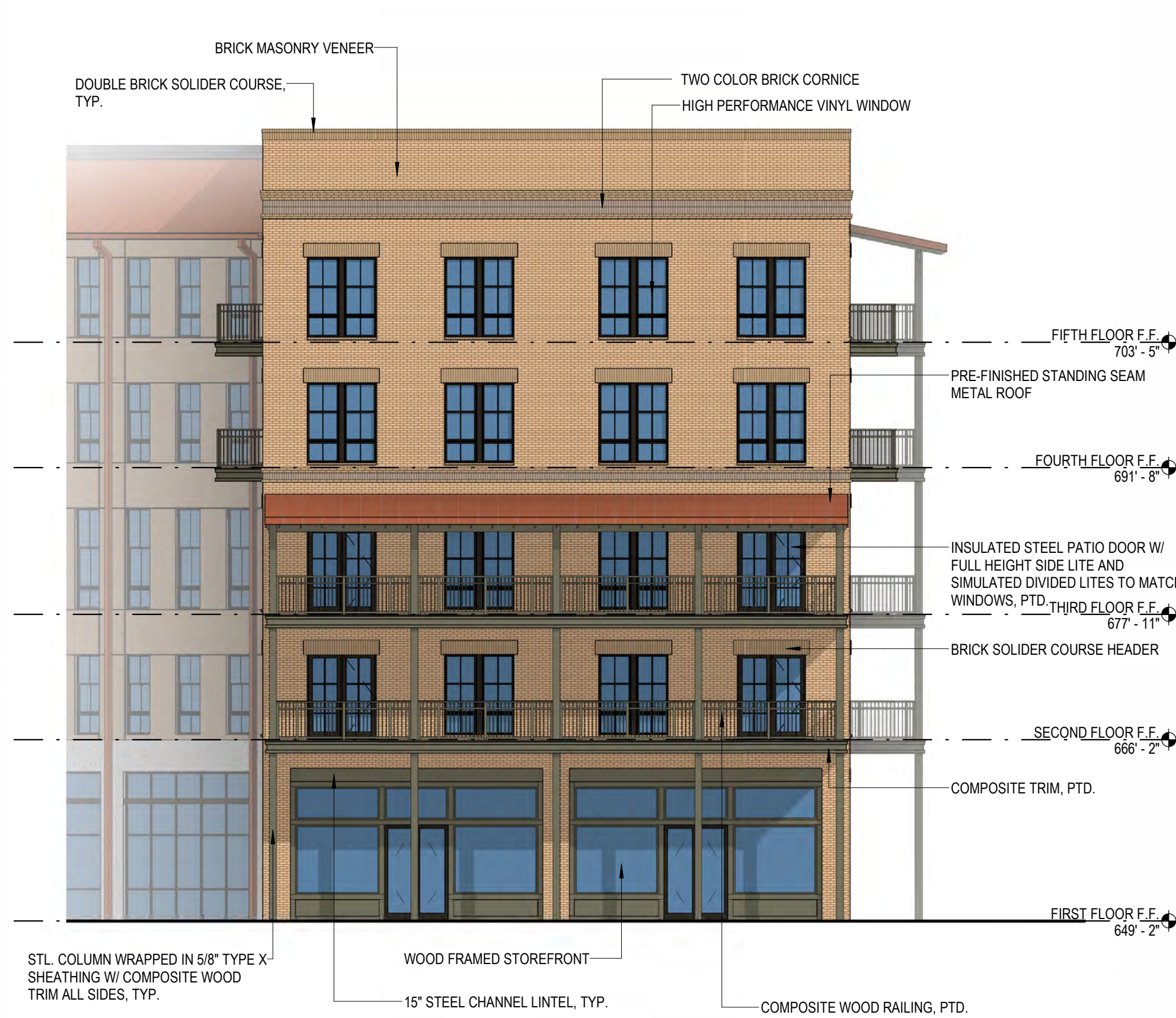
1 ALAMO ST. BUILDING - EXTERIOR ELEVATION - NORTHWEST 3/32" = 1'-0"
