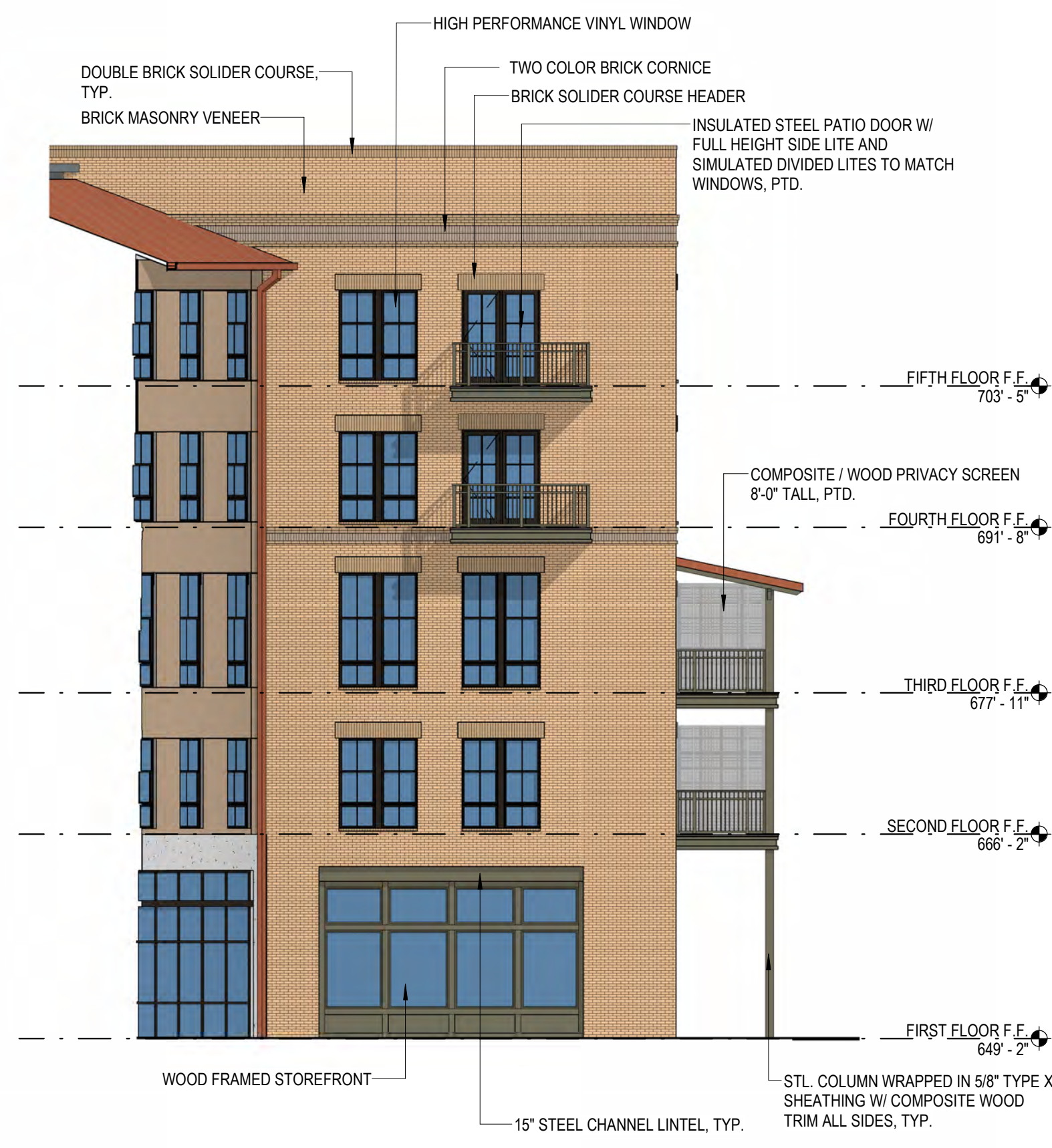
2 ALAMO ST. BUILDING - EXTERIOR ELEVATION - NORTHEAST 3/32" = 1'-0"
