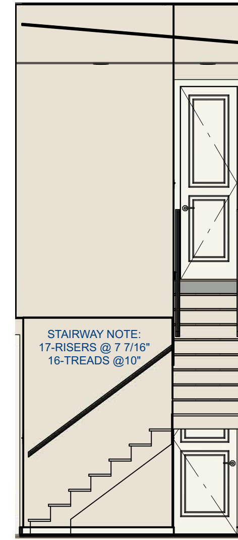
3 STAIRWAY DETAIL 2 SCALE: 1/4"=1'-0"
