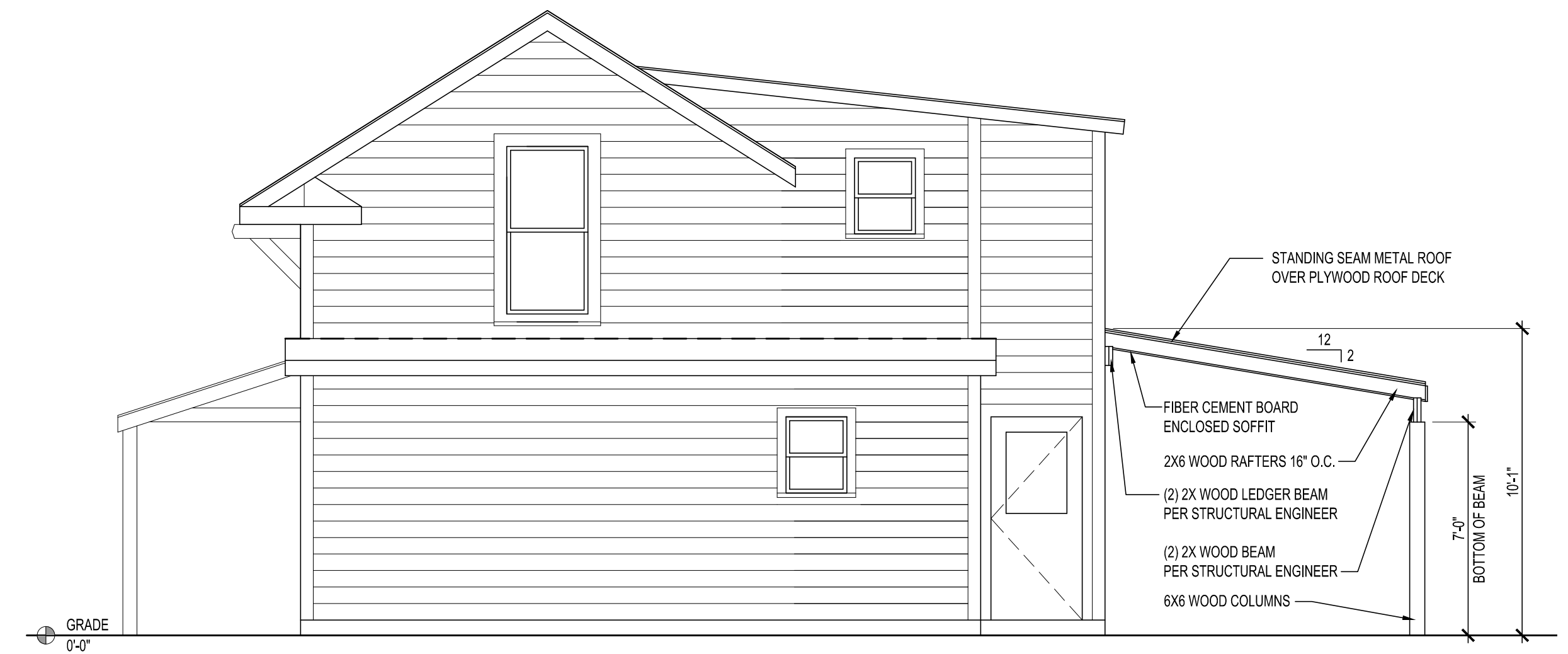
6 CASITA CARPORT - WEST ELEVATION SCALE: 1/4" = 1'-0"
